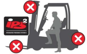
IPS2 includes an electronic parking brake which is applied automatically if the seat is empty. In addition, this can be done manually via a dashboard button.
